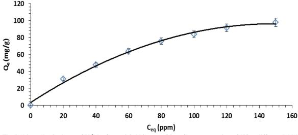
Fig. 5. Adsorption isotherm of Pb<sup>2+</sup> by freeze-dried biomass of *Pseudomonas aeruginosa* 2103 at different initial concentrations.
