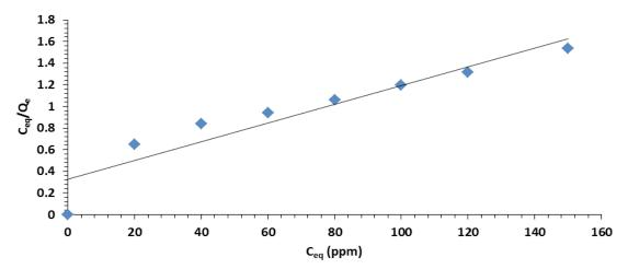
Fig. 6. The linear form of the Langmuir adsorption isotherm of Pb<sup>2+</sup> by freeze-dried biomass of *Pseudomonas* aeruginosa 2103.
