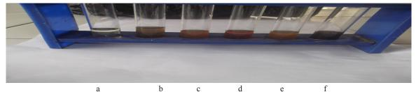
Fig. 6. Effect of different concentration of silver nitrate on production of nanosilver particules at: (a) Without any metals, (b) 0.1mM, (c) 0.2mM, (d) 0.5mM, (e) 1mM, and (f) 2mM.
